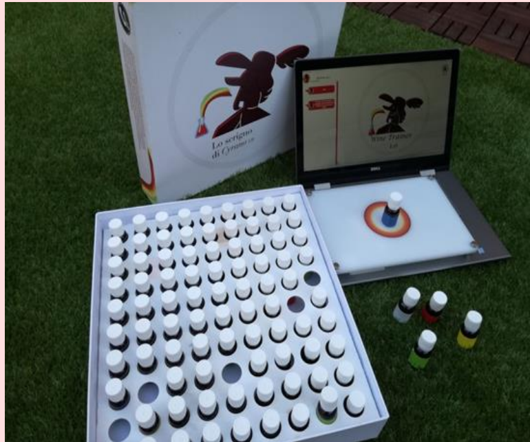
Figure 1: Mergo KIT adapted from the Aromaster kit. Each smelling jar is recognized by an Android smartphone using the MERGO app.
